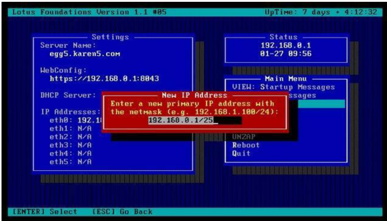
Figure 10. Setting the IP address from the Lotus Foundations server console
