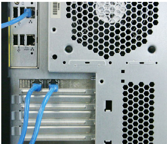
Figure 8. View of Ethernet ports 1 and 2
