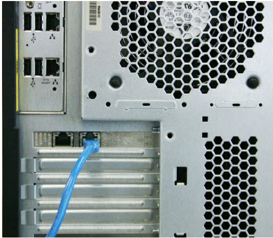
Figure 7. View of Ethernet port 0
